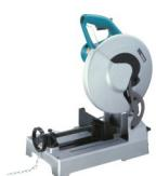
15 amps. 1300 RPM. Cuts 4-1/2" at 90" and 3-1/2" at 45". Carbide tipped blade lasts 50X longer & cuts 4X faster than abrasive blades. Leaves metal bur free and cool to touch. Weighs 42.5lbs
