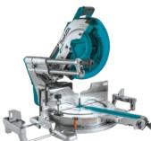
4400 RP electronically controlled. Max cut: 3-5/8x15 at 90°, vertical cut 6-3/4" and crown mold 8 nested. Miters 0-60° left and right; bevels 48° left and right. Up to 175 cuts per charge in 2x12. Weighs 74lbs with battery.
