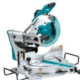
15 amps. 3200 RPM. Soft start, electronic speed control. Built -in laser. 6-5/8" nested crown molding cutting capacity. Cuts 2-13/16"x12" at 90° and 2-13/16"x8-1/2" at 45°. Operation flush against wall. Weighs 57lbs
