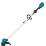
3 speed: 4000, 5000, 6000 RPM. Over heat warning system indicator with automatic shut-off. 11-3/4" cutting capacity. Reverse rotation to clear trimmer head. Weighs 8.6lbs with battery and 72-1/2" long. Bump feed trimmer head. Uses 1—18 volt battery
