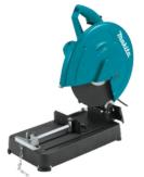
15 amps. 3800 RPM. Cuts 5' round or 4x7-5/8 rectangle at 90" . Abrasive blade with 1" arbor. Tool-less vice adjustment. Weighs 37lbs
