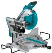
4400 RP electronically controlled. Max cut: 2-13/16x12 at 90°, vertical cut 5-1/4" and crown mold 6-5/8 nested. Miters 0-60° left and right; bevels 48° left and right. Up to 334 cuts per charge in 2x4 and 192 cuts in 2x12. Weighs 60lbs with battery.
