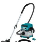
120CFM suction and 44" of water lift with batteries. 3 stage HEPA filtration. Self cleanin filter system. 2.1 gal container. Up to 80min run using 2-18 volt batteries Weighs 17.8lbs with battery
