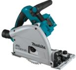
2500-6300 RPM. w/ electric brake. LED battery indicator. 48° max bevel. 2-3/16" max cut at 90° and 1-9/16" max cut at 45°. Weighs 11.2lbs with batteries. 13-5/8" long. Uses 2-18 volt batteries
