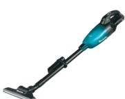
4 speed. Up to 64 min of run time with a 2ah battery . 42 CFM and 84" static water lift. 2 stage HEPA filter. Weighs 4.3lbs with battery
